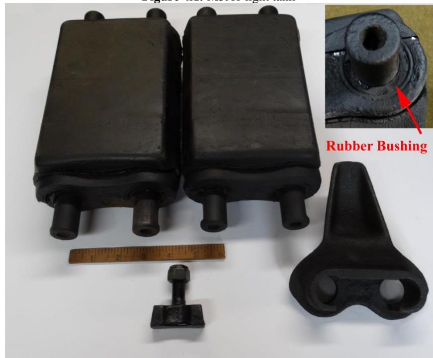
Figure 4B: Two track sections, connector guide and wedge lock fastener
