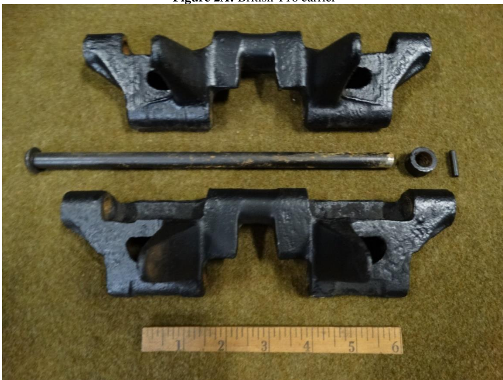
Figure 2B: Two track sections with pin, donut retainer and roll pin
