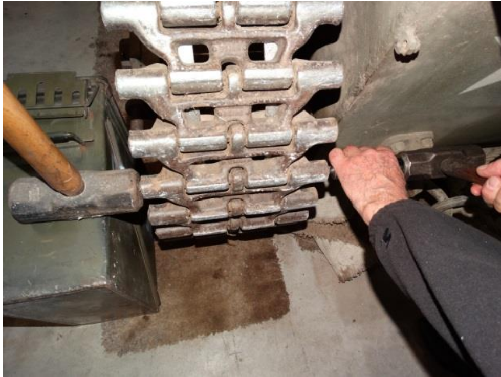
Figure 1C: Staking the retainer onto the track pin
