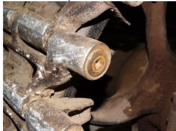
Figure 1D: View of pin head end and staked end
