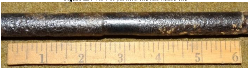
Figure 1E: Wear pattern in the center with pitting corrosion to the left and right
