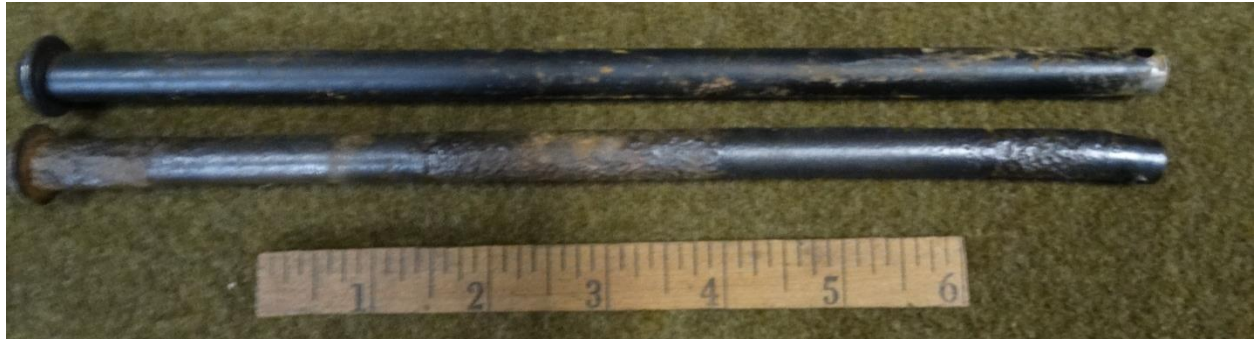
Figure 2C: New upper pin and used lower pin showing wear and pitting corrosion patterns
