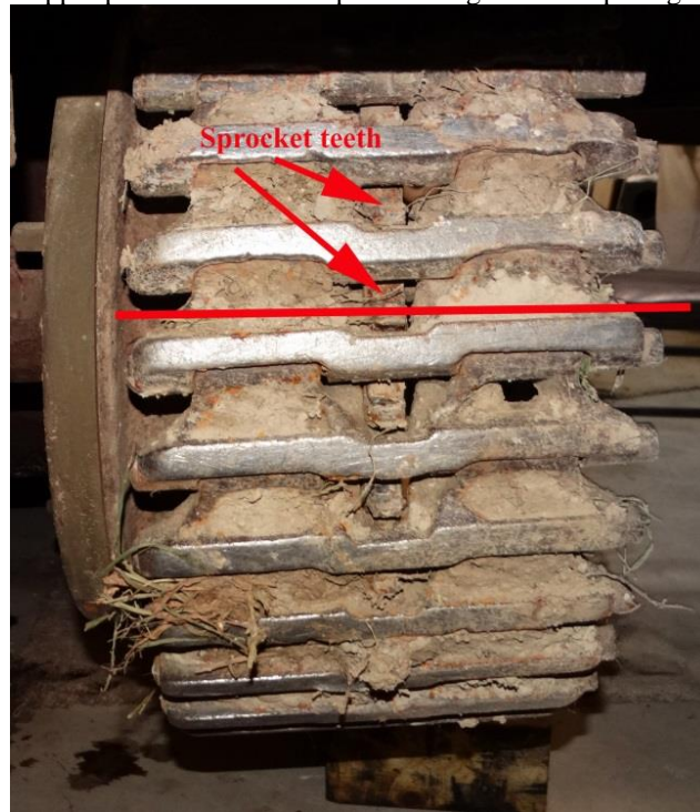
Figure 2D: Track twist from excessive wear and bending of track pins
