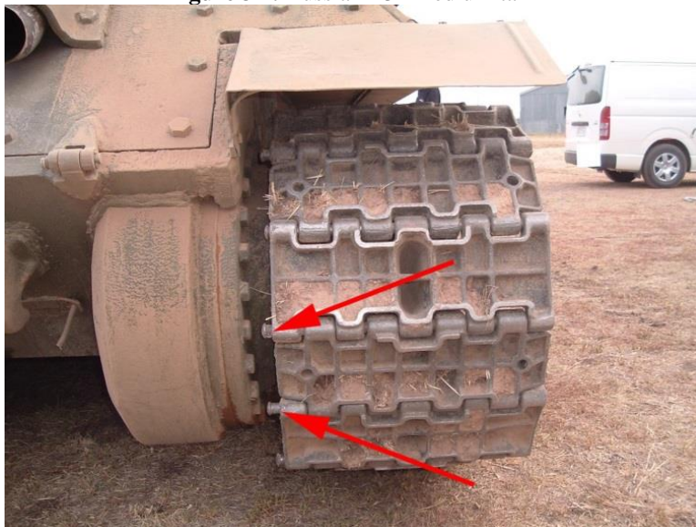
Figure 3B: Track pins working out of position in a T34 (Courtesy of Doug's Heavy Metal Gallery)
