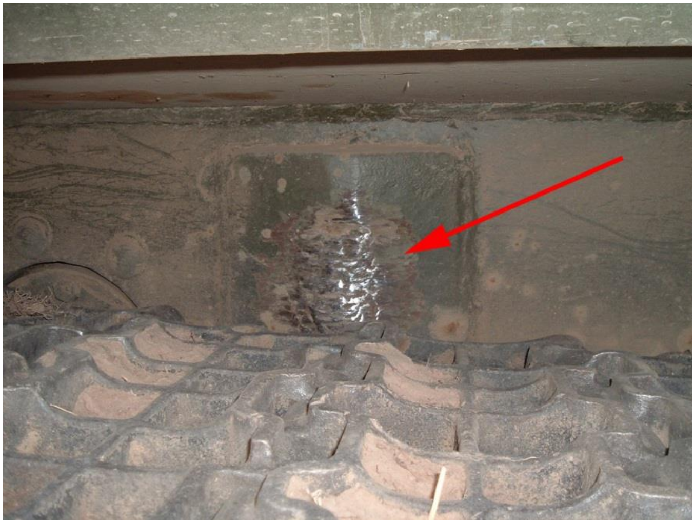
Figure 3C: Track pin shoulder pin relocater welded on the side of the hull (Courtesy of Doug's Heavy Metal Gallery)
